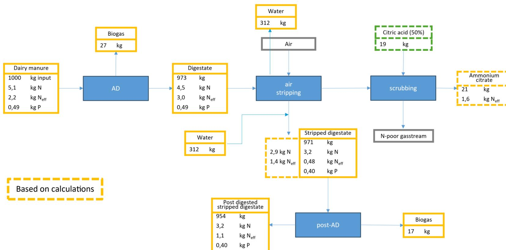
**Figure 10. Cascade 1 – mass- and nutrient balance implementing post anaerobic digestion and nitrogen recovery from dairy manure.**
