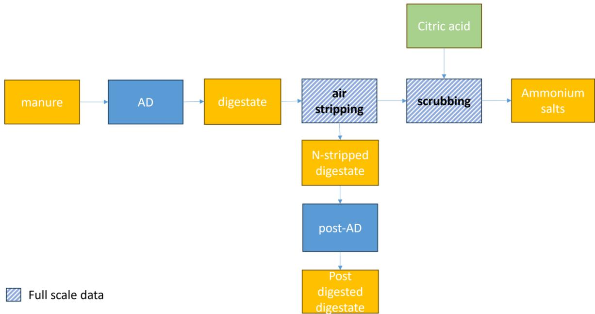
**Figure 2. Cascade 1 – post anaerobic digestion and nitrogen recovery from dairy manure.**
