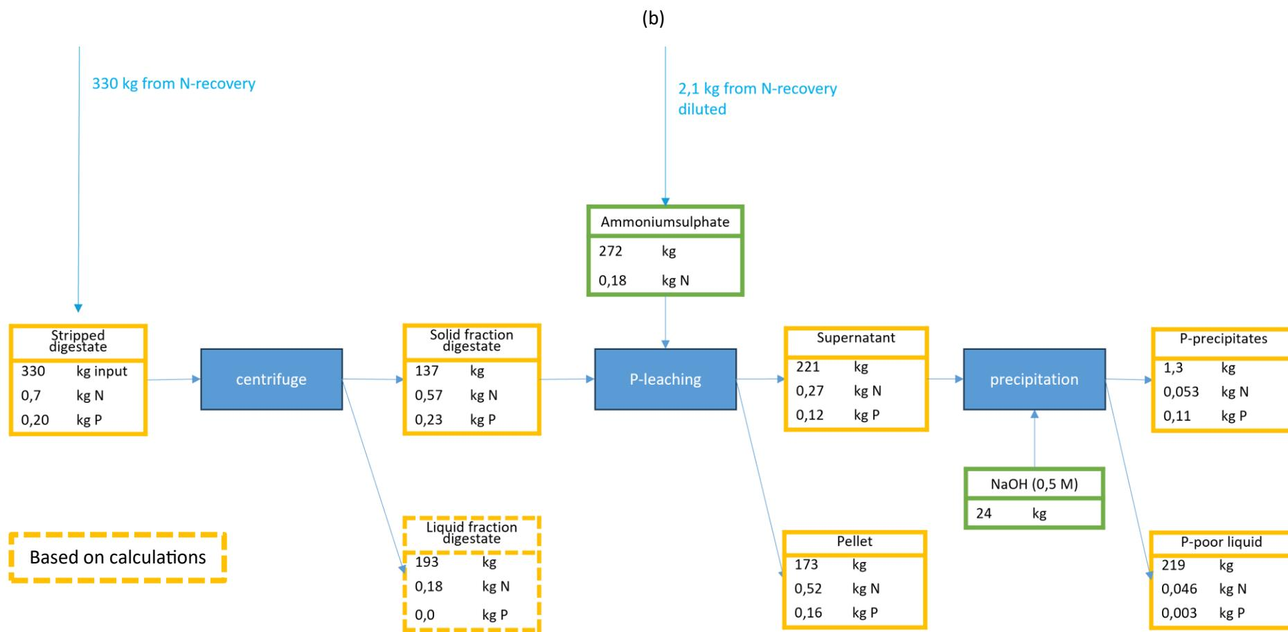
**Figure 12. Cascade 3 – mass and nutrient balance implementing (a) post-anaerobic digestion and nitrogen recovery coupled with (b) phosphorus recovery from dairy manure.**
