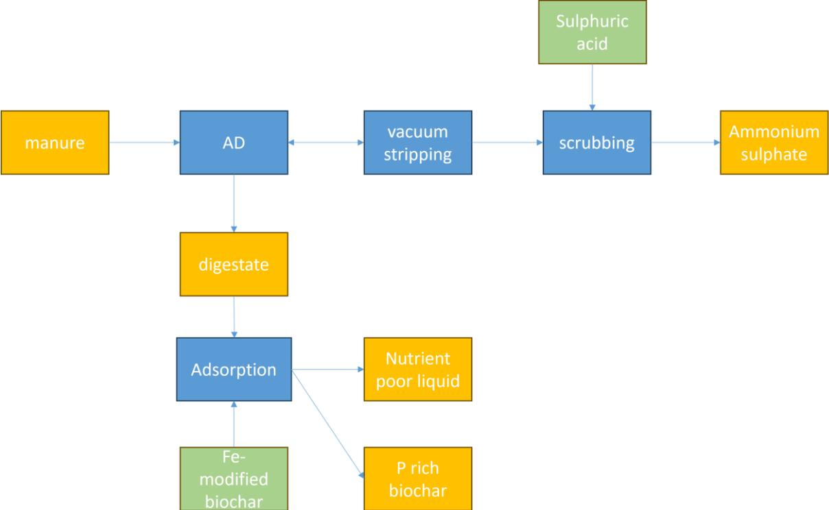
Figure 7. Cascade 6 – nitrogen recovery and phosphorus recovery on Fe-modified biochar.
