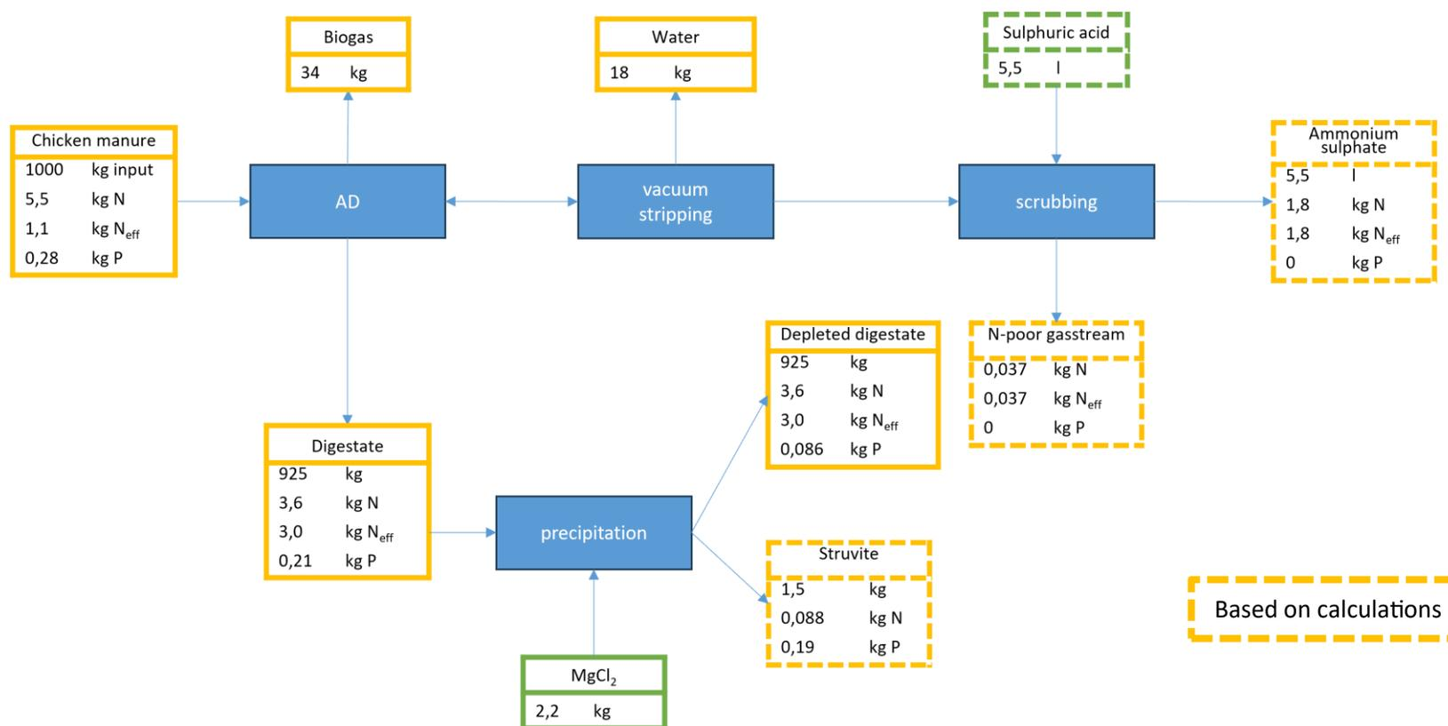
**Figure 14. Cascade 5 – mass and nutrient balance implementing vacuum stripping, nitrogen recovery, and phosphorus recovery as struvite.**
