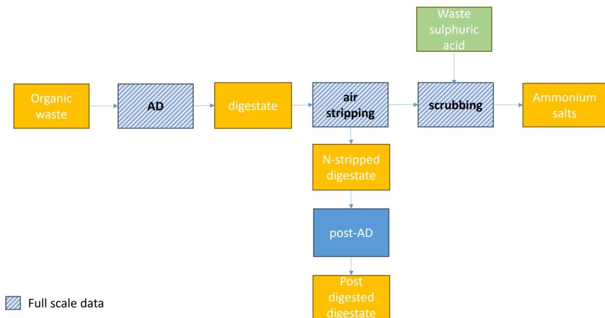
**Figure 5. Cascade 4 – post anaerobic digestion and nitrogen recovery from mixed organic waste.**
