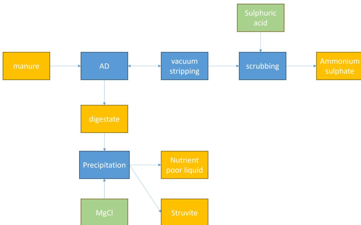
**Figure 6. Cascade 5 – nitrogen recovery and phosphorus recovery as struvite.**
