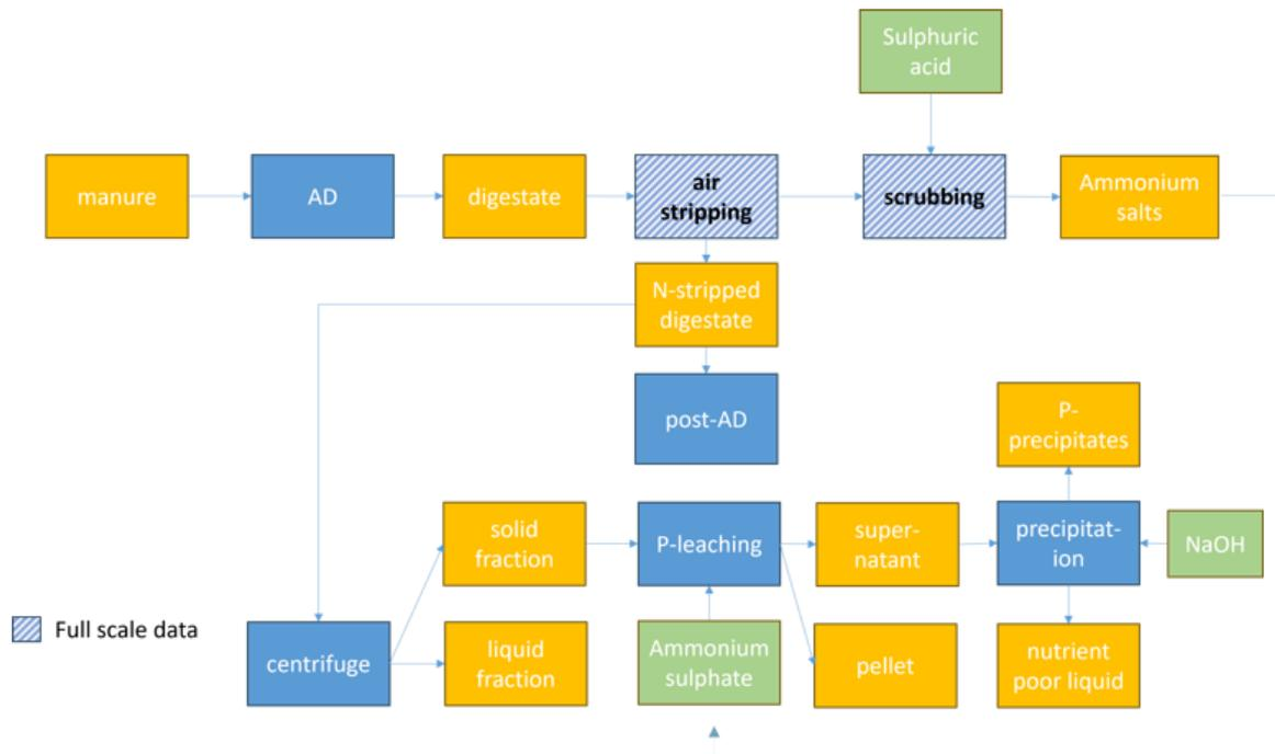
**Figure 4. Cascade 3 – post anaerobic digestion, nitrogen, and phosphorus recovery from dairy manure.**
