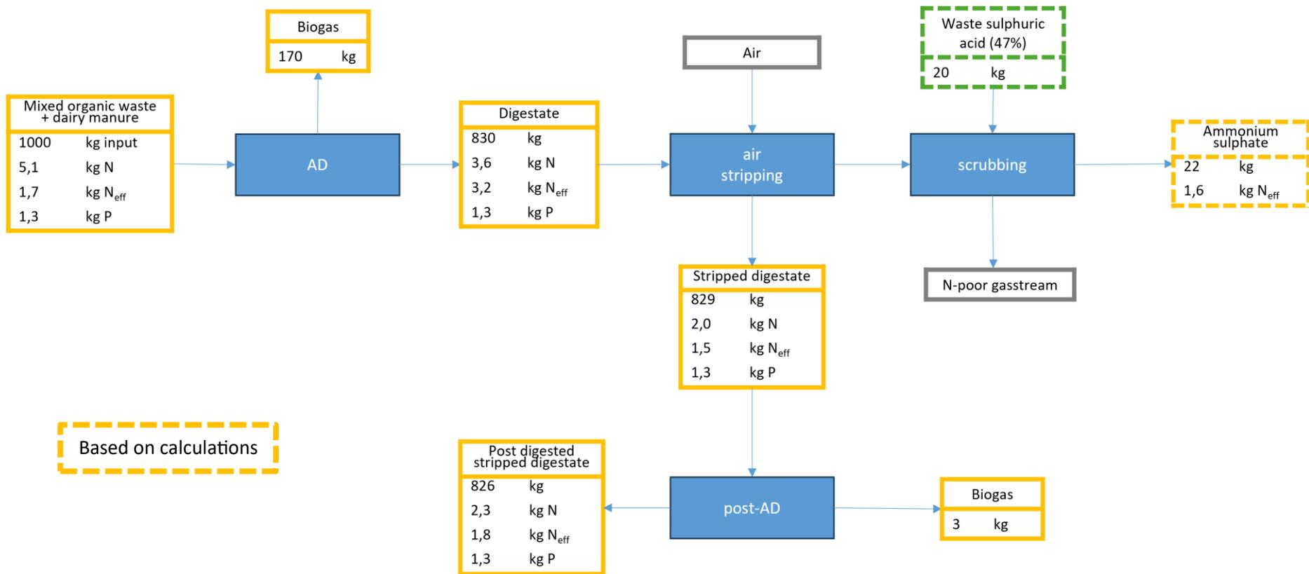
Figure 13. Cascade 4 – mass and nutrient balance implementing post-anaerobic digestion and nitrogen recovery from mixed organic waste and dairy manure.
