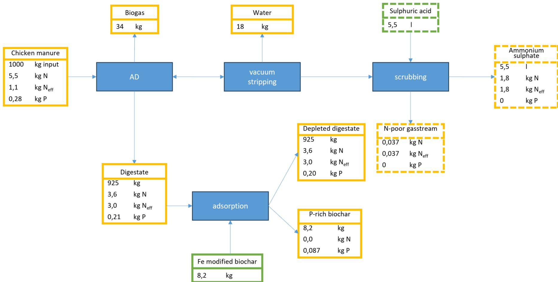
Figure 15. Cascade 6 – mass and nutrient balance implementing vacuum stripping, nitrogen recovery, and phosphorus recovery on Fe-modified biochar.
