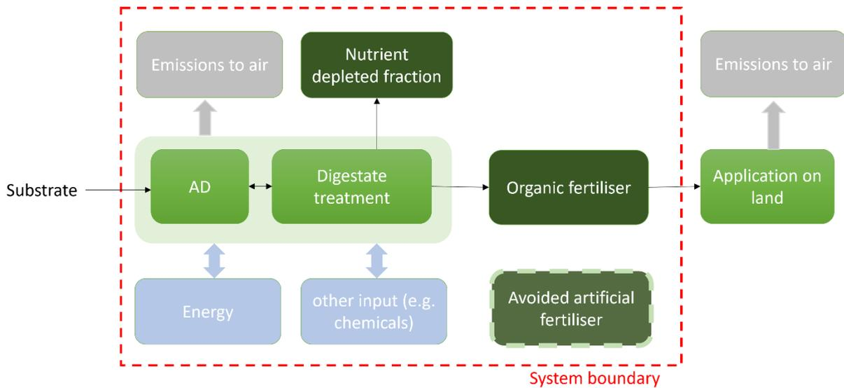
**Figure 17. Generalized scheme of emissions related to the different technology cascades.** The red dashed line represents the system boundary.
