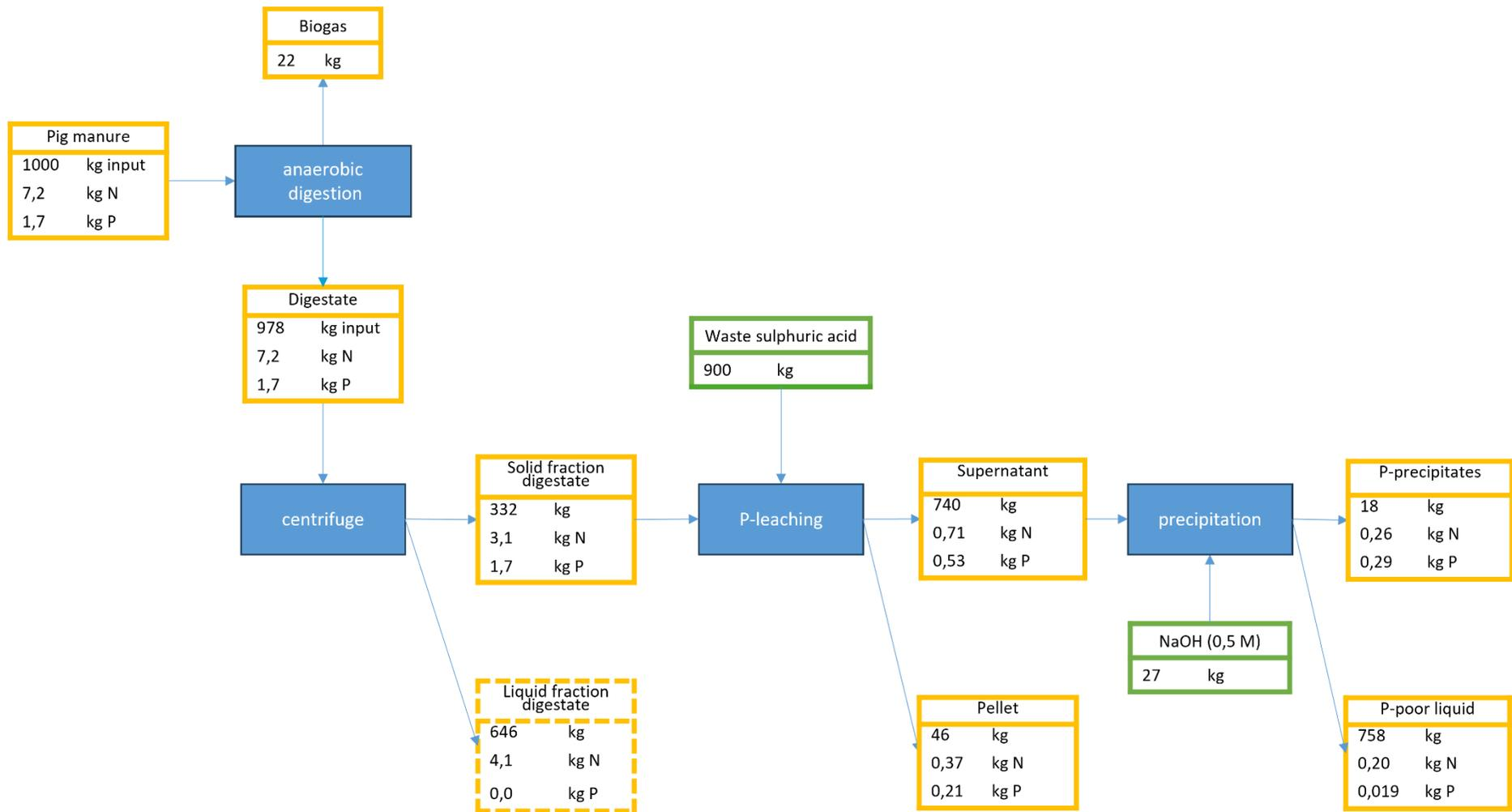
Figure 11. Cascade 2 - mass and nutrient balance implementing phosphorus recovery from pig manure.
