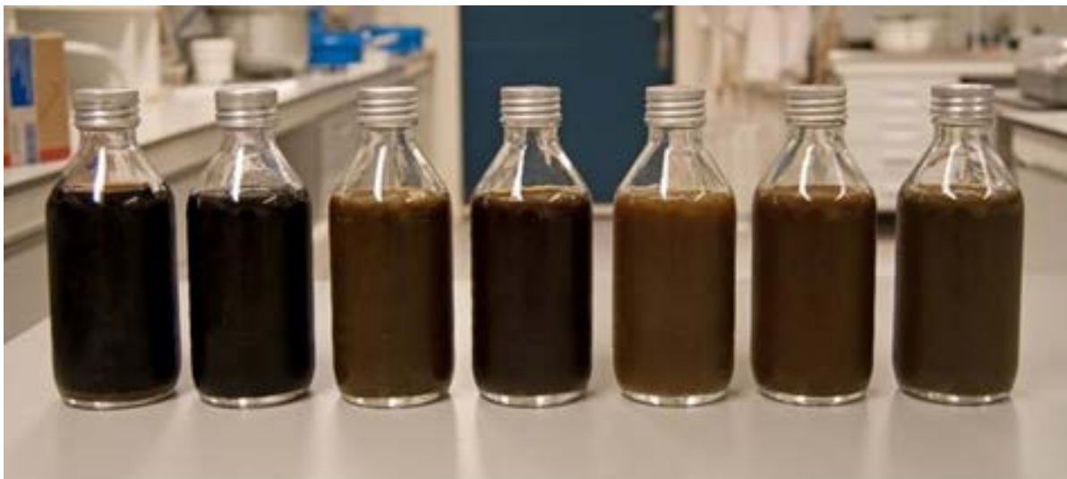
Figure 12: Samples of mineral concentrate of different reverse osmosis installations.
